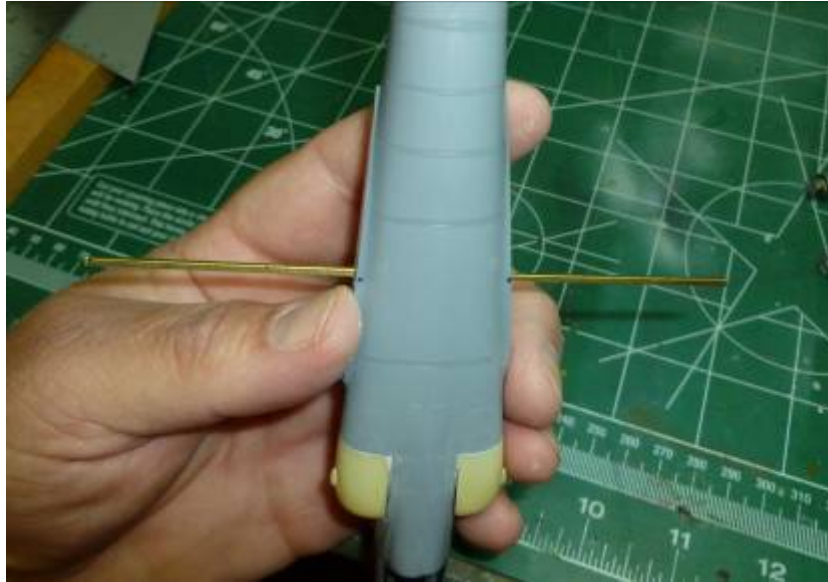
Photo 2: The wing spar. I have already re-scribed the fuselage panel lines at the joint. They have been brushed with Extra Thin and will be buffed once dry.
