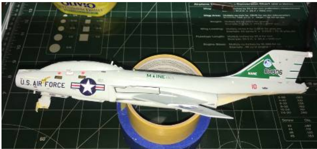
Photo 16: Enlisting gravity to lend a hand. Note how the nose strut was masked during painting.
