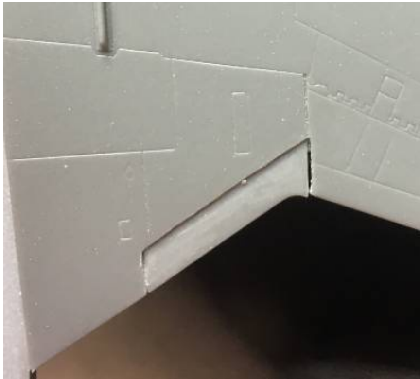
Photo 7: The upper flap gap and step.
