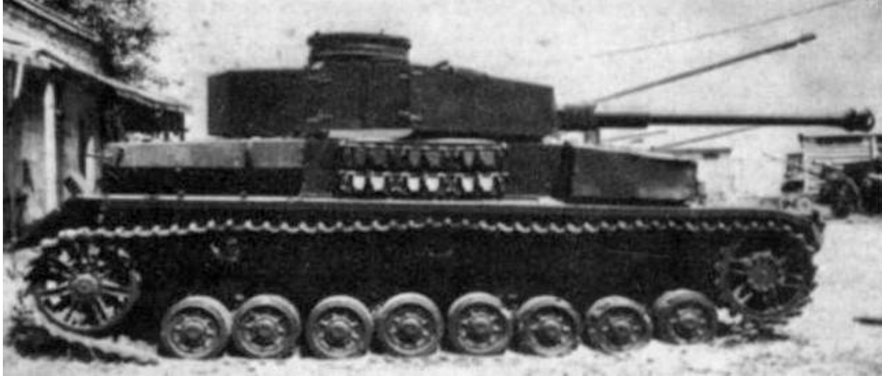
Panzer IV Ausf H of the Syrian army. The spare tread links were both a breakdown recovery item, and added a bit of extra armor for the crew. A few links were carried on the right side, and more on the front glacis.
