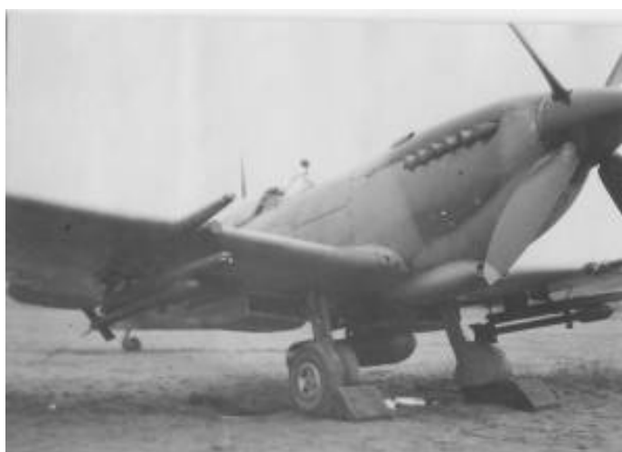
Photo 13: 74 Squadron Spitfire IXe armed with rocket projectiles. (RAF via 74 Sqn Association)
