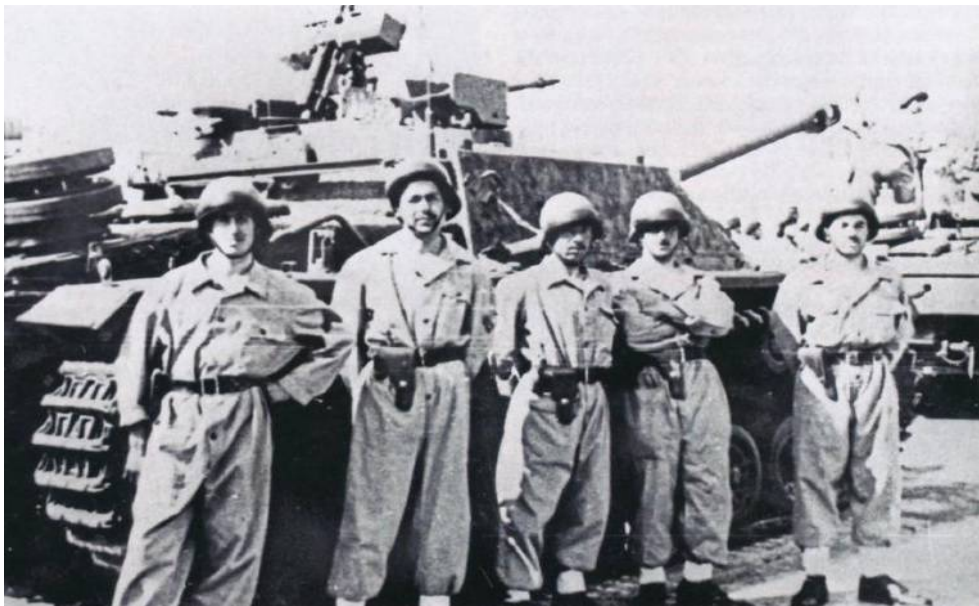
Syrian army StuG III in the early 1960s. This shows the SAFAT mount in addition to the WWII-standard MG-34 mount.
