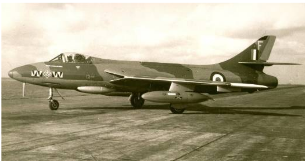
Photo 22: A 74 Sqn Hawker Hunter F.4. Note the straight wing leading edge. (RAF via 74 Sqn Association)
