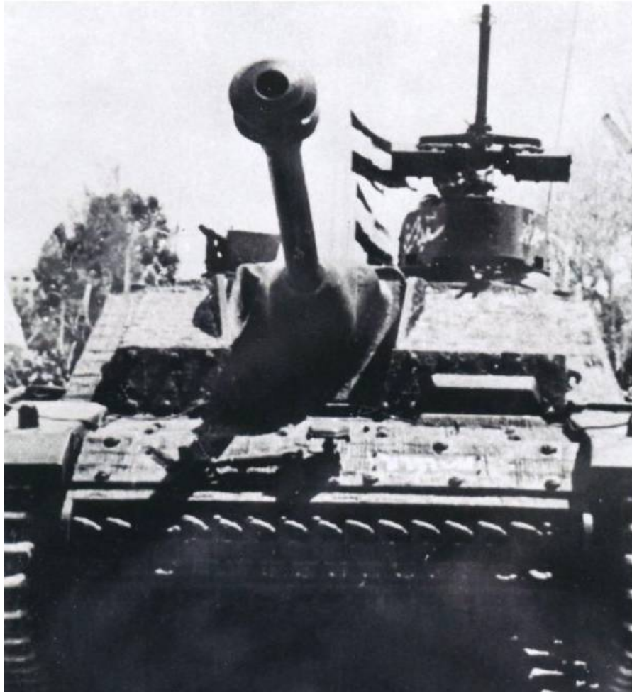
Syrian StuG III in the early 1960s with the locally-designed mount for the Italian SAFAT machine gun. Also of note, this StuG still has the WWII German "Zimmerit" anti-magnetic coating on; it can be seen clearly around the area scraped clean for the Syrian serial number. Zimmerit was a paste which tended to come off over time.
