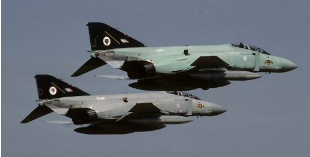
Photo 32: A good photo showing the color differences between the NARF paint on "Juliet" (foreground) and proper RAF colors on "Oscar" (farthest from camera). (Colin Collis via 74 Sqn Association)
