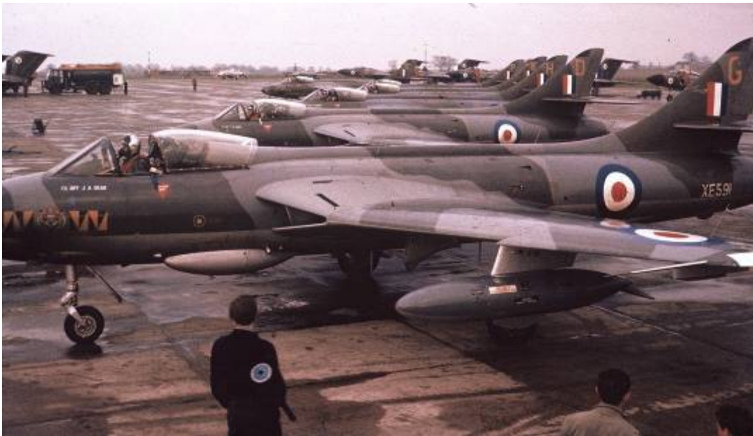
Photo 24: A Hunter F.6 on a rapid turn-around. Note the dogtooth on the wing leading edge. (RAF via 74 Sqn Association)
