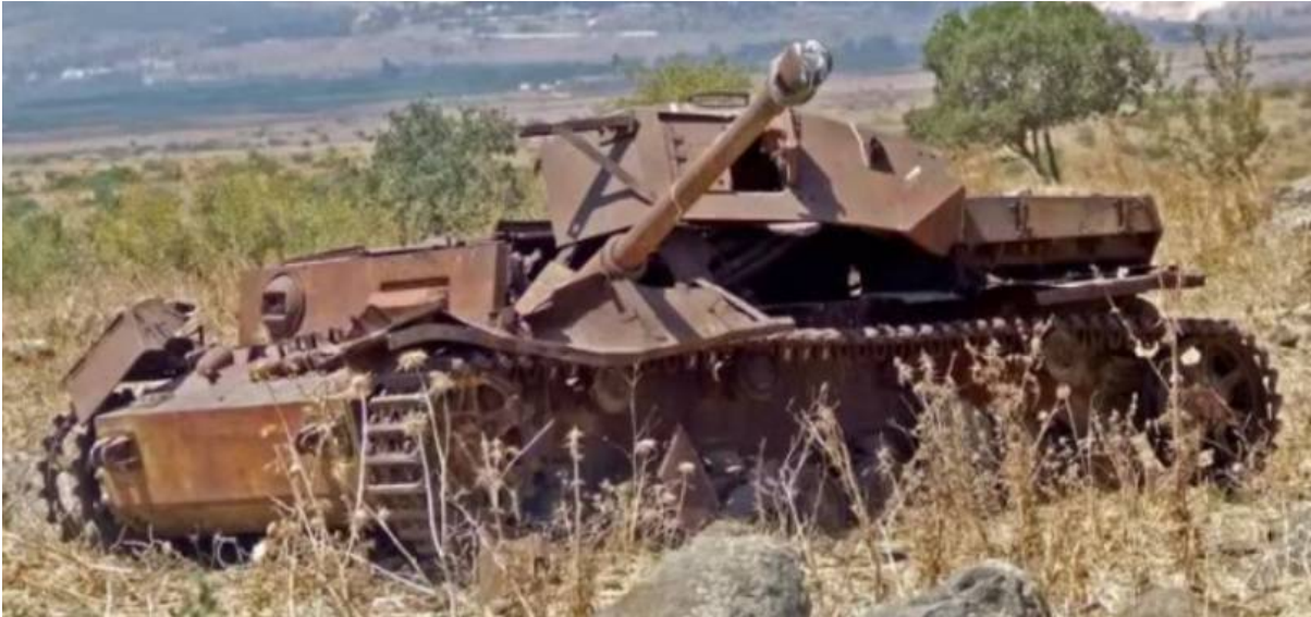
This Syrian Panzer IV near Mt. Hermon was “racked” (suffered a penetrating hit resulting in it’s ammunition exploding) during the Six Day War.
