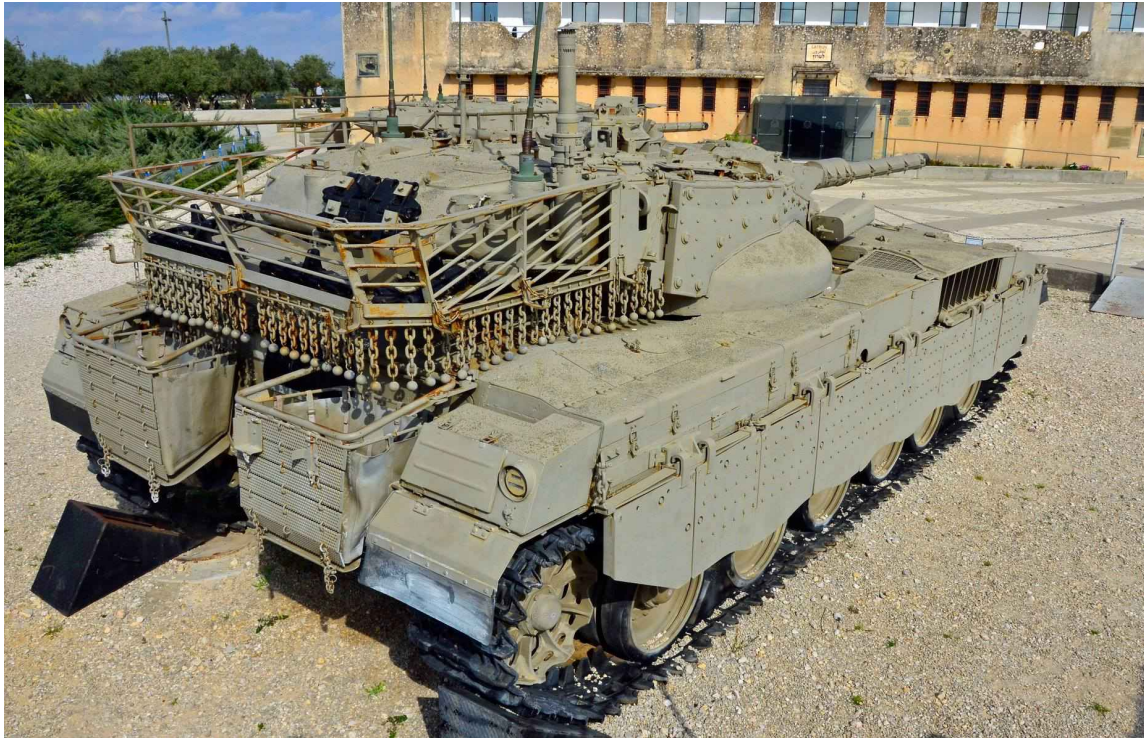
Merkava Mk.II from the rear. Note the distinctive "Ball and Chain" protecting the shot trap in the rear of the turret from RPGs.
