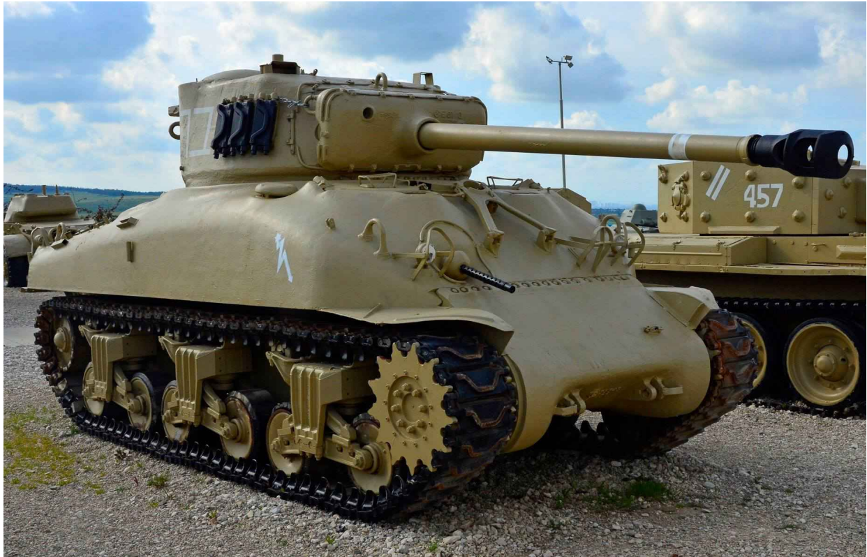
Sherman M-50, a Sherman tank upgraded with a French 75mm gun from their AMX-13
