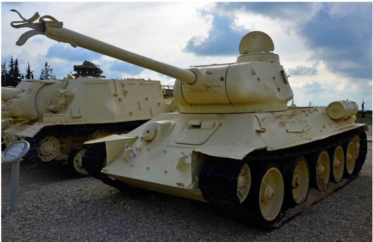
T-34 85 with a burst barrel
