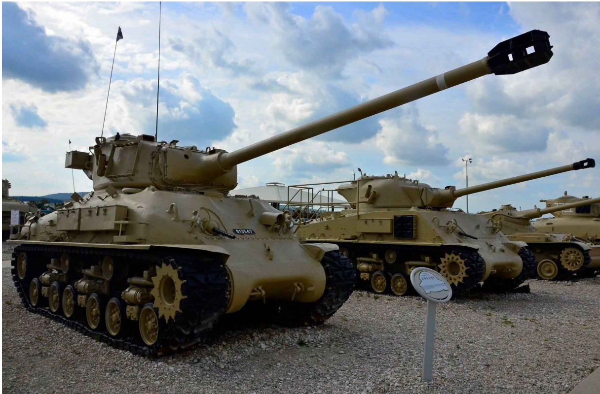
Sherman M-51 with a French 105mm gun from the AMX-30. Note the muzzle brake
